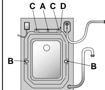
2) Unscrew the two rods **B** and remove them. N° 2 or N° 4 plastic spacers will fall inside the machine.
