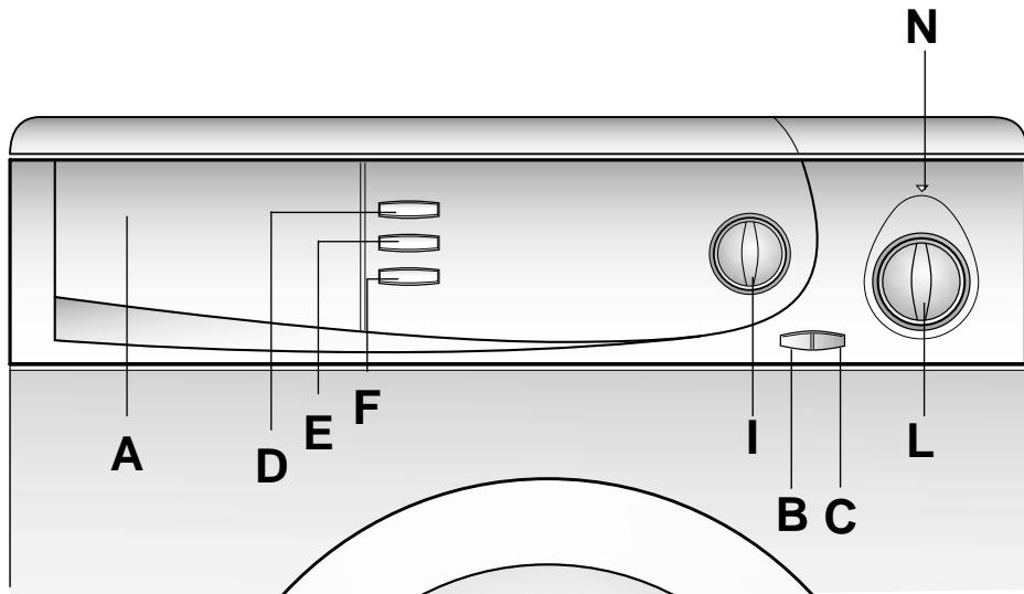
**CONTROLS***Detergent drawer**Door open button**Off/On button**800/400 button**Extra Rinse button**No spin button**Wash control temperature knob**Timer knob for wash programmes**Off/On indicator light*A
